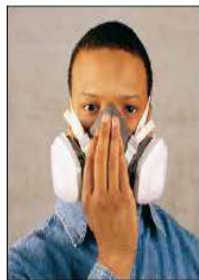
Place the palm of your hand over the exhalation valve cover and exhale gently. The facepiece should bulge slightly. If air leaks between the face and the faceseal, reposition it and adjust the straps for a more secure seal.
