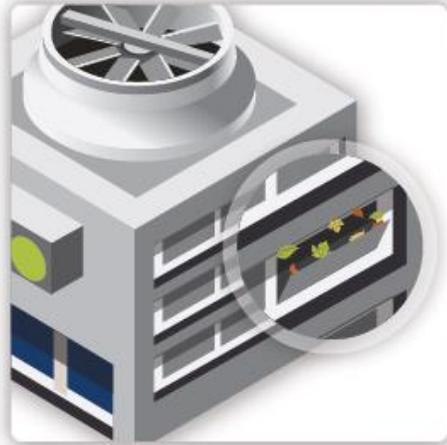
1. During weekly inspection of the cooling tower, Michelle discovers that leaf litter has accumulated in the reservoir.
